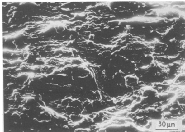
Figure 12 SEM fractography of overload region for 23TAHA1 specimen.
