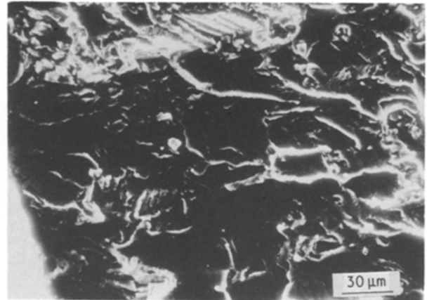
Figure 9 SEM fatigue fractography for OTHA1 specimen.
